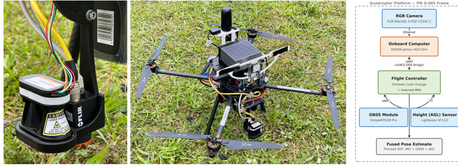
Fig. 4: Hardware configuration. Left: Nadir-pointing RGB camera FLIR Blackfly S-PGE-31S4C-C [15] and the height AGL sensor Lightware SF11/C [28]. Center: Quadcopter PM Q-685 [36] custom frame, equipped with NVIDIA Jetson AGX Orin [41], GNSS module SimpleRTK2B Pro [2], and flight controller Pixhawk Cube Orange with its IMUs [46]. Right: Block diagram of the SafeLand hardware setup.
